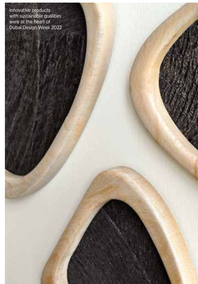
Palm veneer is made up of pressed palm fibres
